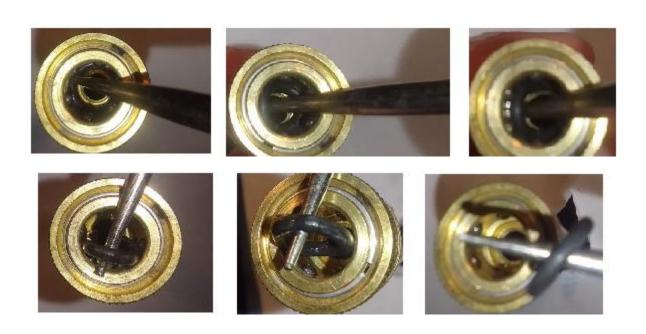
To install a new O-ring in the quick coupler, pinch the O-ring between your fingers and insert it into the coupler.
